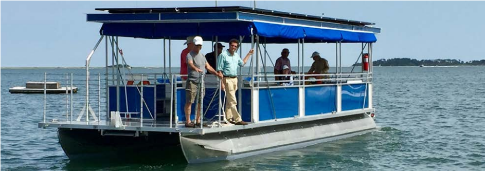
"The Friend" – New 37' Solar Electric Pontoon Boat for educational and research activities in the greater Pleasant Bay estuary on Cape Cod.
