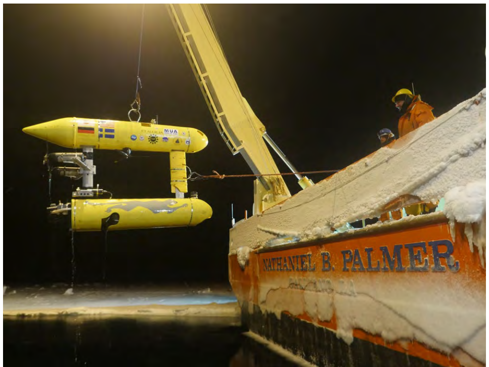
The author deploying WHOI's Jaguar AUV on a mission under the Antarctic sea ice to measure its thickness.
